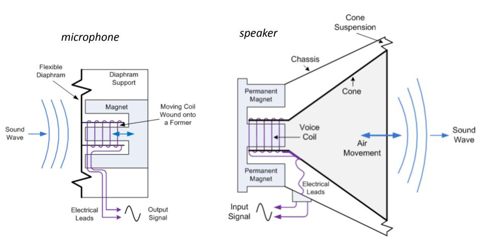
• Note: voice coil can also be used to generate fast motion
